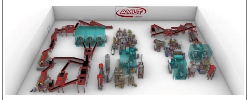
The lines, which will be processing light weight bottles with high percentages of PVC and non PVC shrinkable sleeves, will feature a double De-Labeller configuration. In the first stage the Amut patented De-Labeller performs a dry cleaning action able to detach most of the shrink sleeves labels while the second unit is a wet De-Labeller working as cold pre-washing, allowing to remove contaminants, without damaging the bottles and avoiding to lose the bottles necks during the process.
